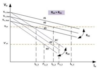
Fig. 2. Load regulation characteristic of droop method
