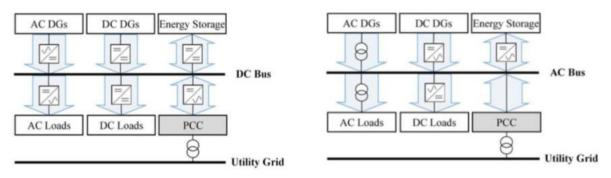
Fig. 1.a) General structure of dc microgrids
