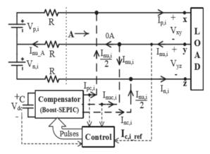
Fig. 3. Circuit with a Boost Sepic converter
